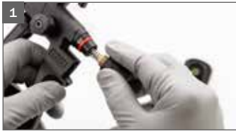
1 First remove paint needle.
