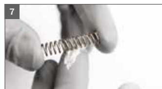
7 Grease and insert paint needle spring
