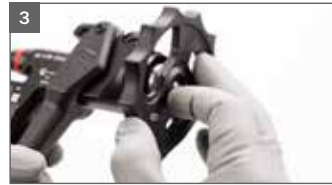
3 Finally, unscrew the paint nozzle using the ring wrench integrated in the universal wrench.
