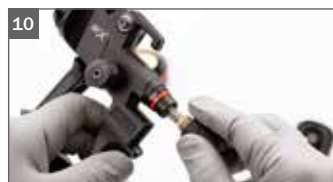
10 Installing material flow regulation screw
